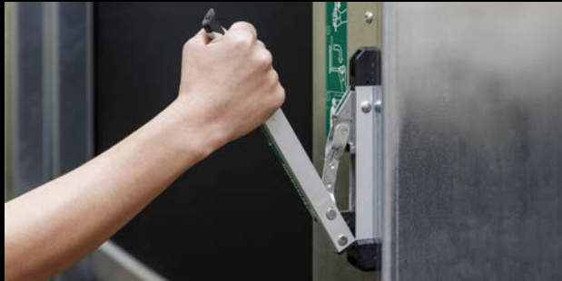
Emergency operation lever
