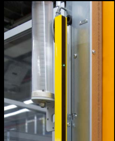
Head-safe option with safety light grid
