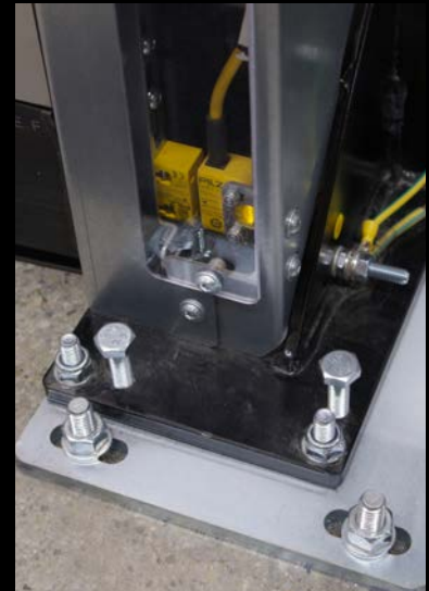
Integrated safety limit switch
