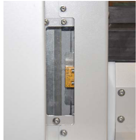
Integrated safety limit switch
