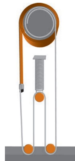
The EFAFLEX wind load system provides permanent door leaf tension. Perfect for wherever the wind or negative pressure can cause draughts!
