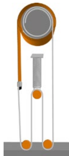
The EFAFLEX wind load system provides permanent door leaf tension. Perfect for wherever the wind or negative pressure can cause draughts!
